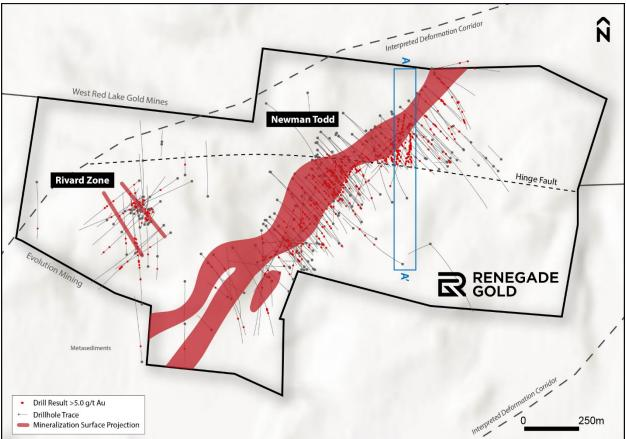
**Figure 1.** *Plan map of the Newman Todd Project showing drilling and modelled gold mineralization projected to surface.*
