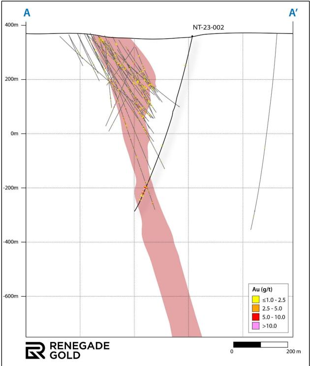
**Figure 2.** Cross section at the Newman Todd Project showing recent step out drilling extending mineralization at depth (NT-23-002).
